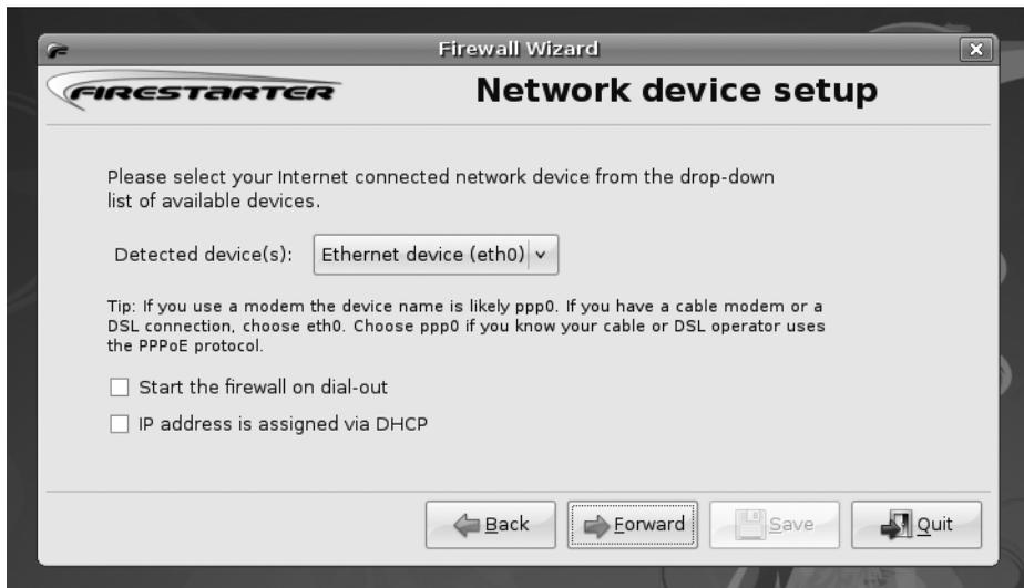
**Figure 9-19.** Firestarter includes a wizard to walk you through the basics of firewall configuration.
