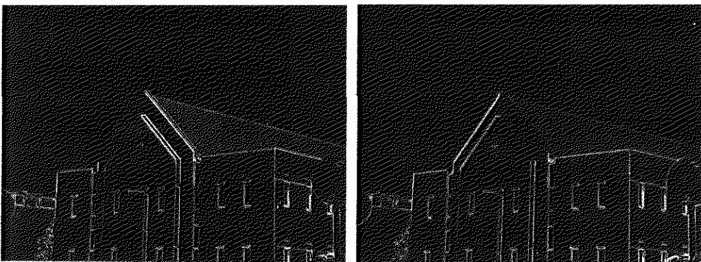
a b FIGURE 10.12 Diagonal edge detection. (a) Result of using the mask in Fig. 10.9(c). (b) Result of using the mask in Fig. 10.9(d). The input in both cases was Fig. 10.11(a).
