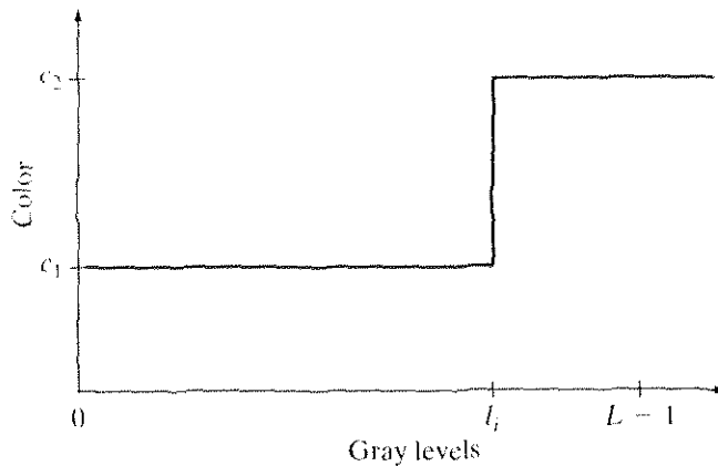
FIGURE 6.19 An alternative representation of the intensity-slicing technique.
