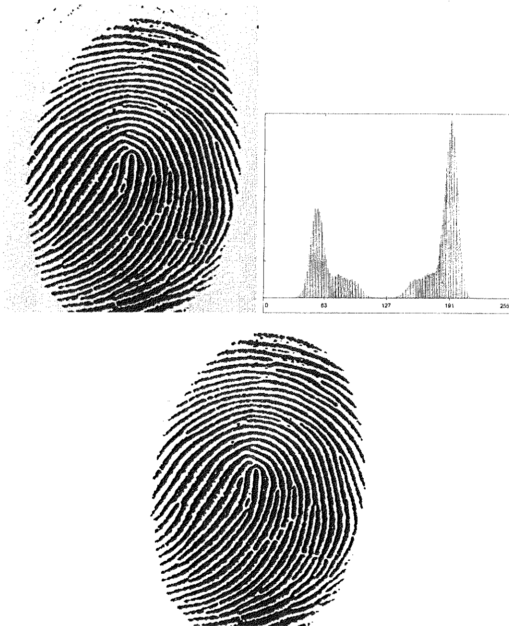
FIGURE 10.29 (a) Original image. (b) Image histogram. (c) Result of segmentation with the threshold estimated by iteration. (Original courtesy of the National Institute of Standards and Technology.)
