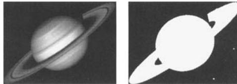
Fig. 7.14 Bimodal Image Thresholding.
